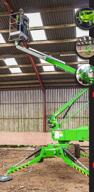
**Highly effective Bi-Energy** system increases flexibility and maximises utilisation in a wider range of environments
